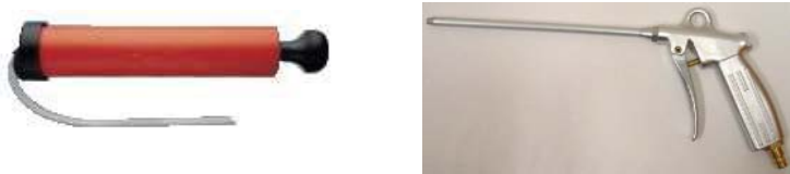
Fig. 1: Setting instructions and necessary cleaning aids (hand pump or compressed air 6 bar)
