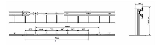
The single-sided vehicle restraint system for installation on driven posts is composed of galvanised components acc. to RAL-RG 620. The lengths of the beams and posts determin the shape of each segment. The system is characterised by its beams of 4 m length and a post spacing of 0,66 m. The joints of the guardrail beams overlap in direction of traffic. They are connected to each other by multiple screwings and fixed to the posts together with the reinforcement beams.
