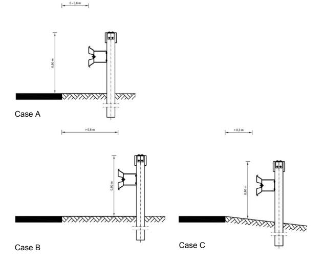
Kerbs with a level difference of more than 7.5 cm should be avoided, level differences of more than 20 cm are not permissible. If kerbs with a maximum height of 20 cm cannot be removed, one of the following solutions should be chosen in consultation with the client:
