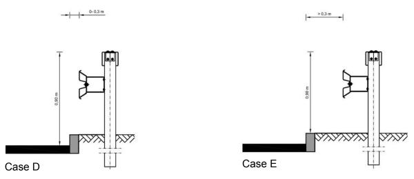
If possible the system should be placed so that the front edge of the guardrail beam is aligned with the front edge of the kerb. In case the distance from the front edge of the kerb is not more than 30 cm (Case D), the installation height is measured from the carriageway surface. In case the distance from the front edge of the kerb is > 30 cm (Case E) the height of the guardrail and box beams is to be measured from the top edge of the kerb.
