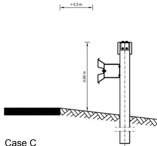
Kerbs with a level difference of more than 7.5 cm should be avoided, level differences of more than 20 cm are not permissible. If kerbs with a maximum height of 20 cm cannot be removed, one of the following solutions should be chosen in consultation with the client:
