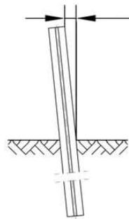
The posts must be driven plumb-vertically. Deviations are permissible up to  $\pm 10\%$  of the total post installation height above ground (that is 8.9 cm deviation at standard installation height). In some cases, individual posts may shift or turn more than 10% due to driving obstacles in the soil (e.g. stones, roots). If this is occurring at more than 20% of the posts, the provisions for driving obstacles outside the defined soil classes apply (see above).
