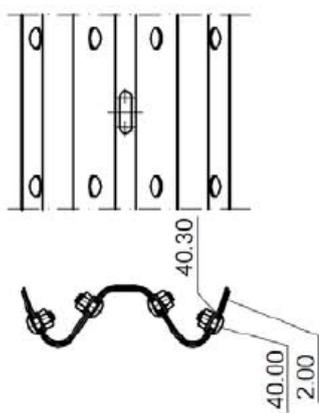
Screwing Beam Joints B-Profile
