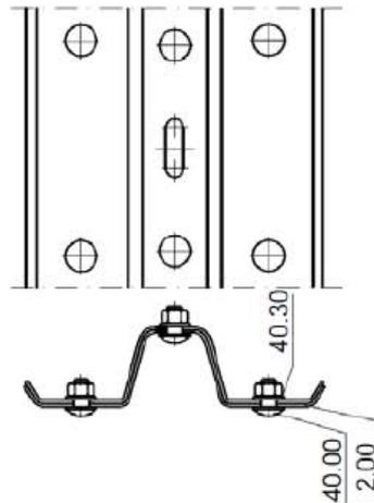
Screwing Box Beam Joints
