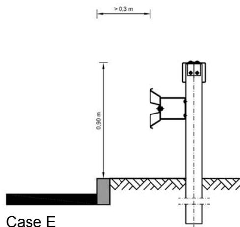
If possible the system should be placed so that the front edge of the guardrail beam is aligned with the front edge of the kerb. In case the distance from the front edge of the kerb is not more than 30 cm (Case D), the installation height is measured from the carriageway
